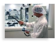
quality. The Q-TRAK™ Plus and IAQ-CALC™ Indoor Air Quality Meters provide powerful solutions using traditional IAQ parameters like temperature, humidity, CO<sub>2</sub>, CO and ventilation rates. The DUSTTRAK™ Aerosol Monitor detects airborne particles from 1 to 10 microns in size, while the P-TRAK™ Ultrafine Particle Counter can track ultrafine particles smaller than 0.1 micron in diameter to their source.
