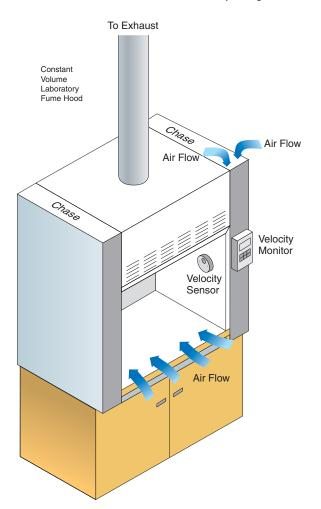
To ensure the safety of your fume hoods, EVERWATCH® Face Velocity Monitors directly measure the average face velocity. TSI's sensor, mounted in the sidewall of the fume hood, detects face velocity disturbances caused by a moving sash, splash shield use, or even a user standing in front of the hood! If the face velocity falls outside of an acceptable range, audible and visual alarms warn users of the unsafe condition.
